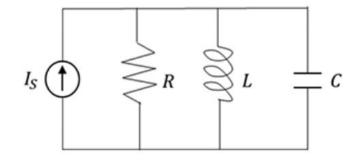
$$Q = \frac{R}{\omega_0 L} = \omega_0 C R = R \sqrt{\frac{C}{L}} \qquad \qquad \omega_0 = \frac{1}{\sqrt{LC}}$$
