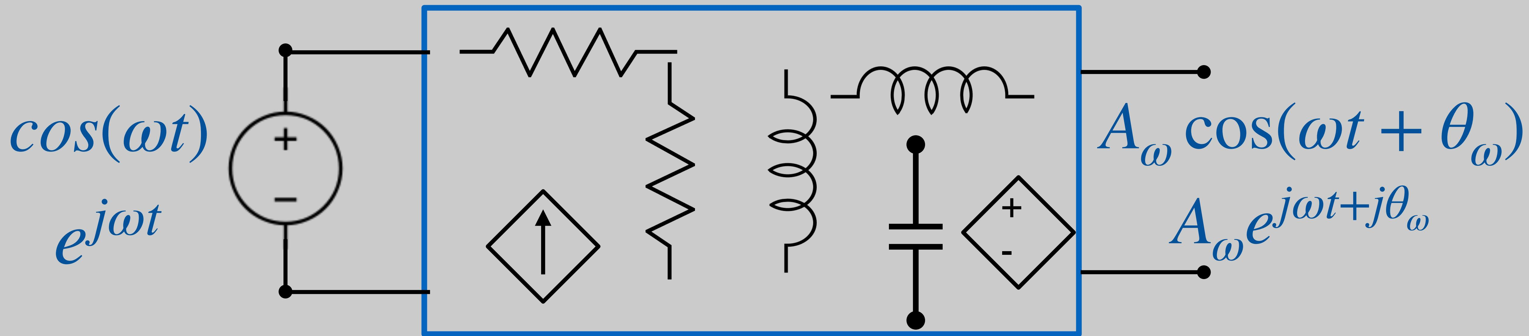
$$H(j\omega) = \frac{A_\omega e^{j\omega t + j\theta_\omega}}{e^{j\omega t}} = A_\omega e^{j\theta_\omega}$$
