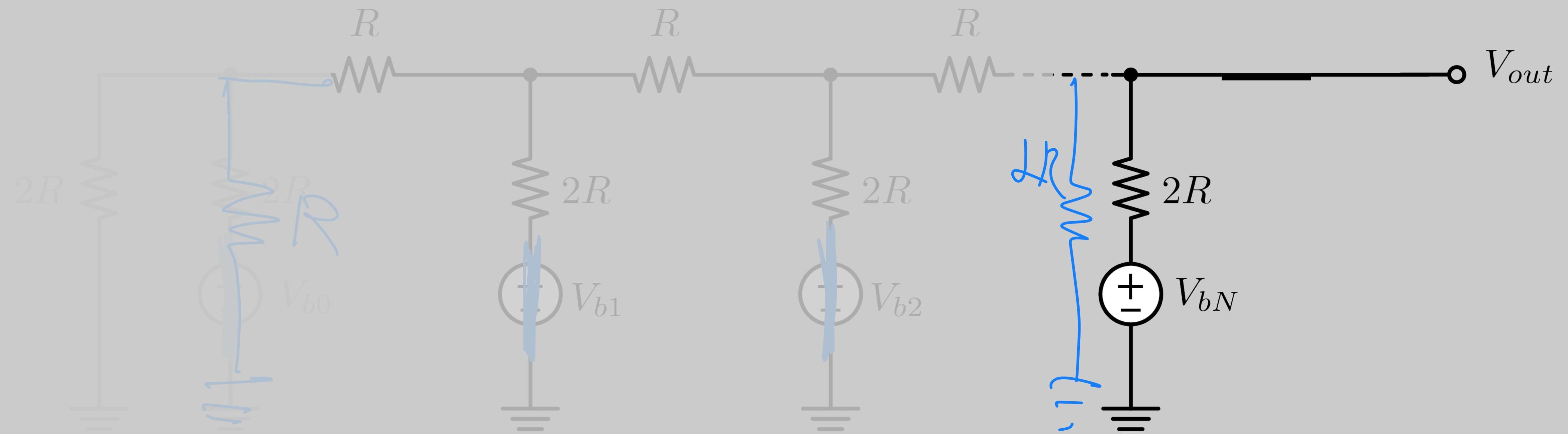
$$V_{out} = \frac{V_{bN}}{2}$$
