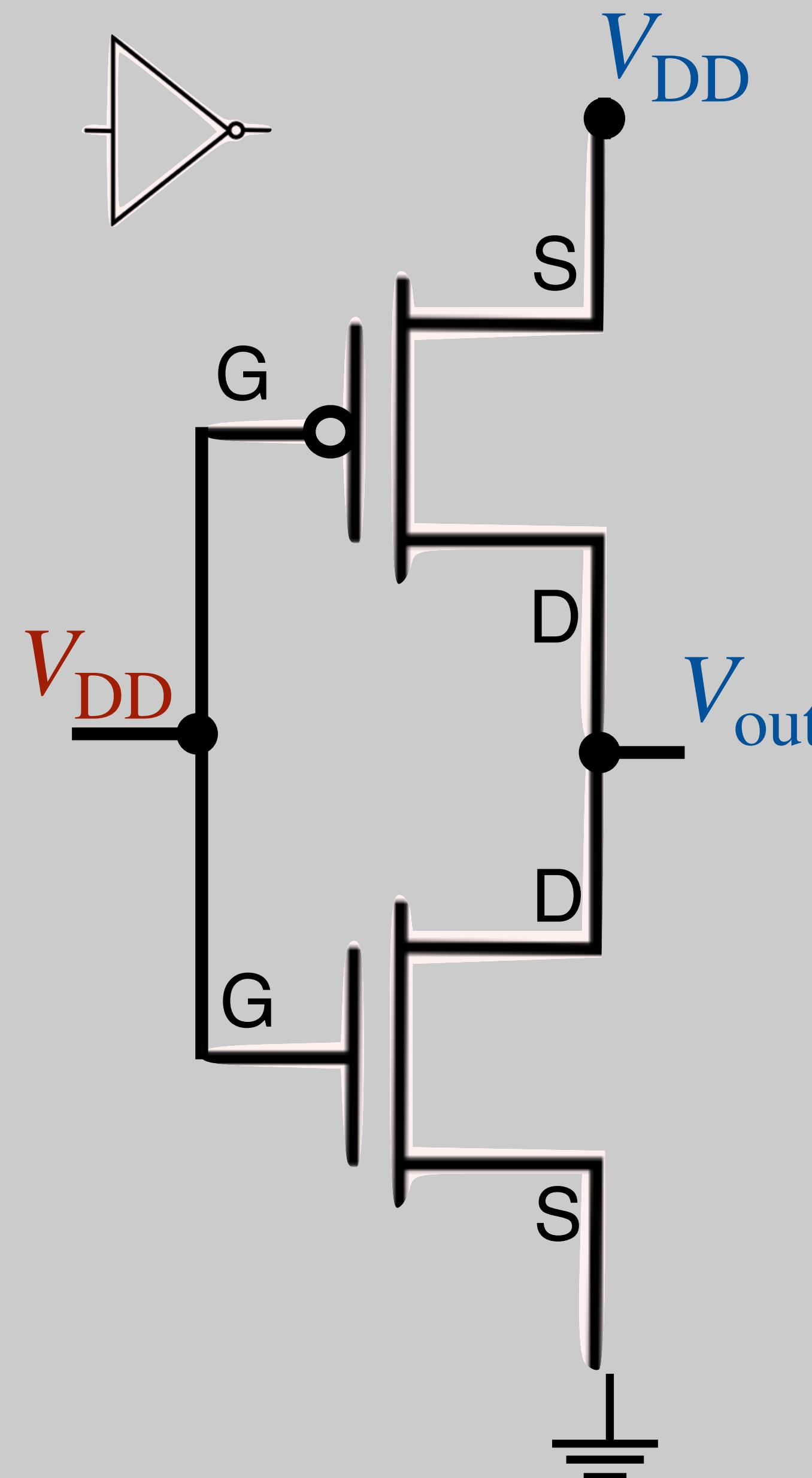
$$V_{in} = V_{DD} \Rightarrow "1"$$
