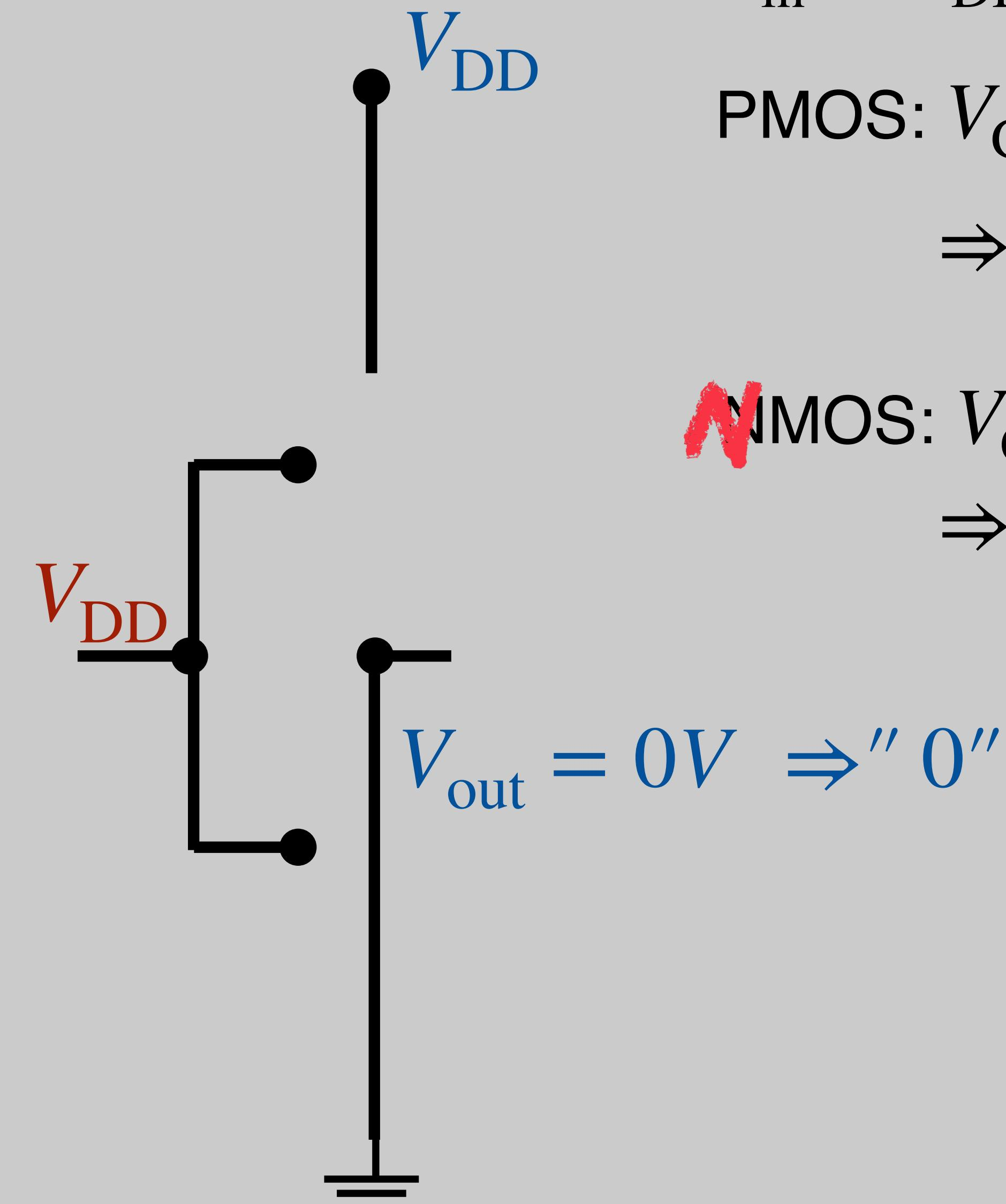
$V_{in} = V_{DD} \Rightarrow "1"$
