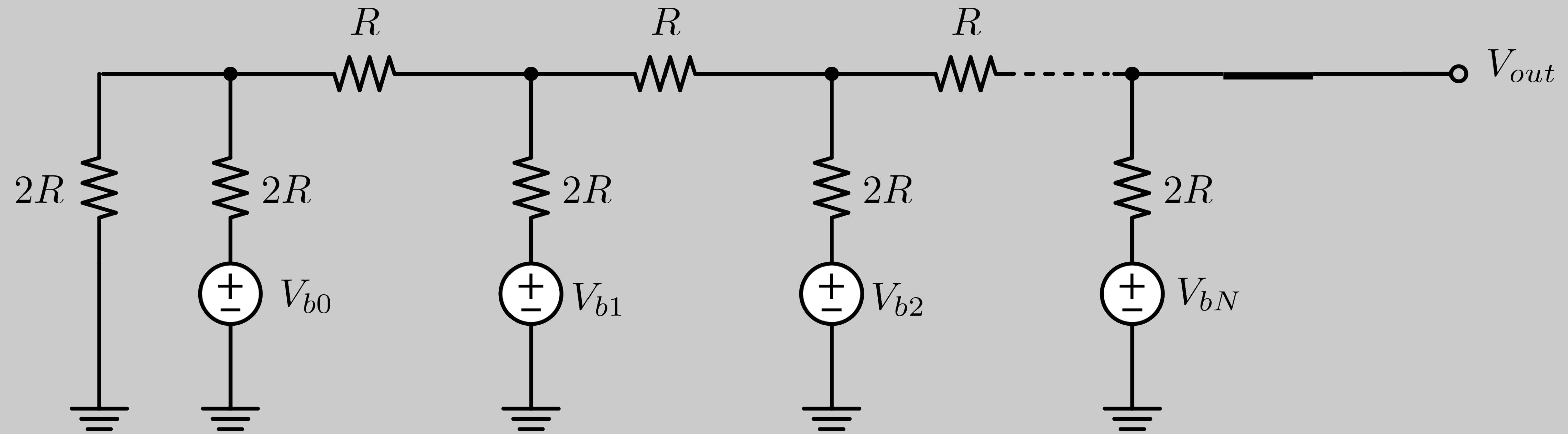
$$V_{out} = \frac{V_{b0}}{2^N} + \frac{V_{b1}}{2^{N-1}} + \dots + \frac{V_{bN}}{2}$$
