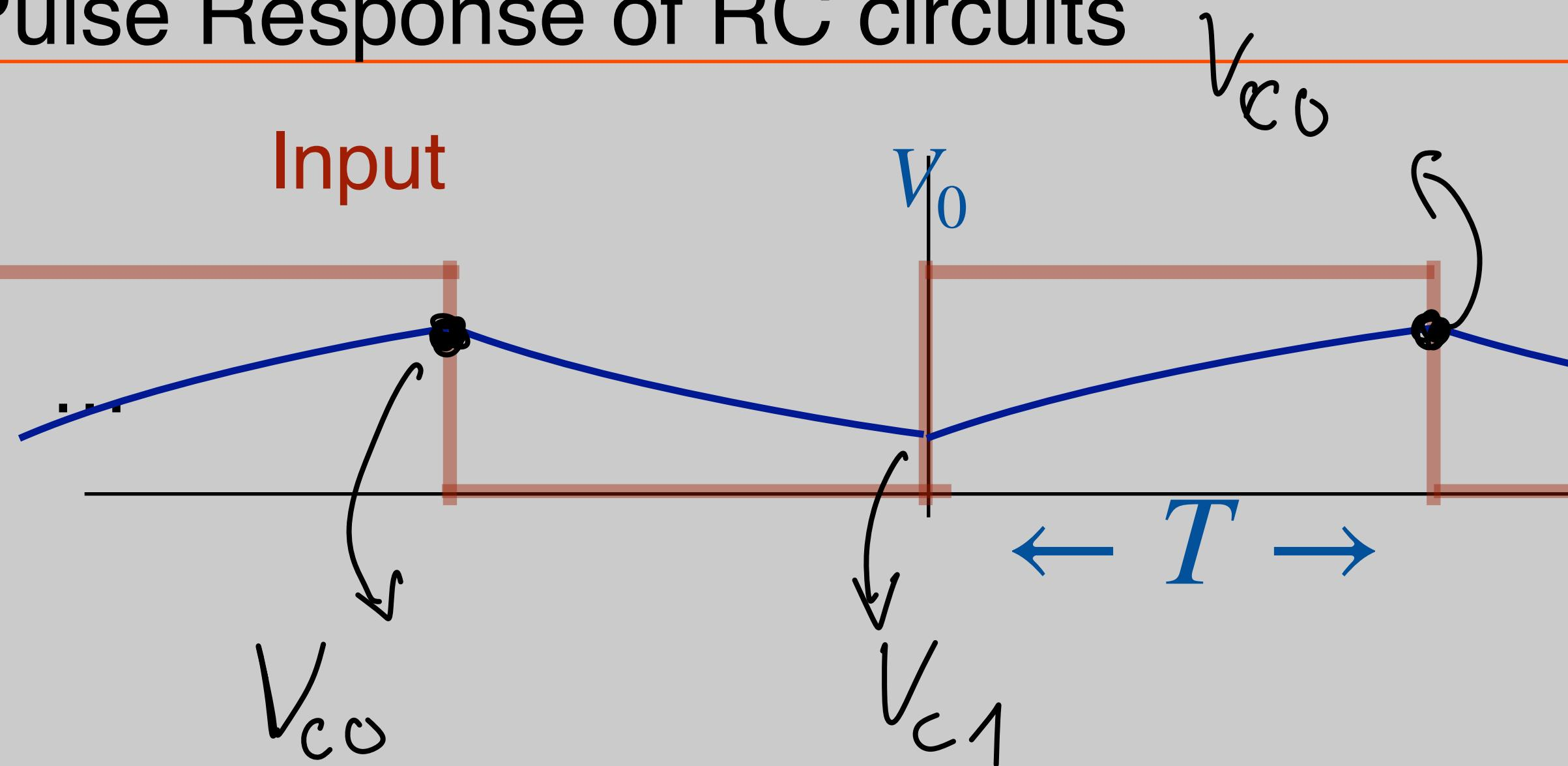
$$\textcircled{1} \quad V_{C1} = V_{C0} e^{-\frac{T}{RC}}$$
