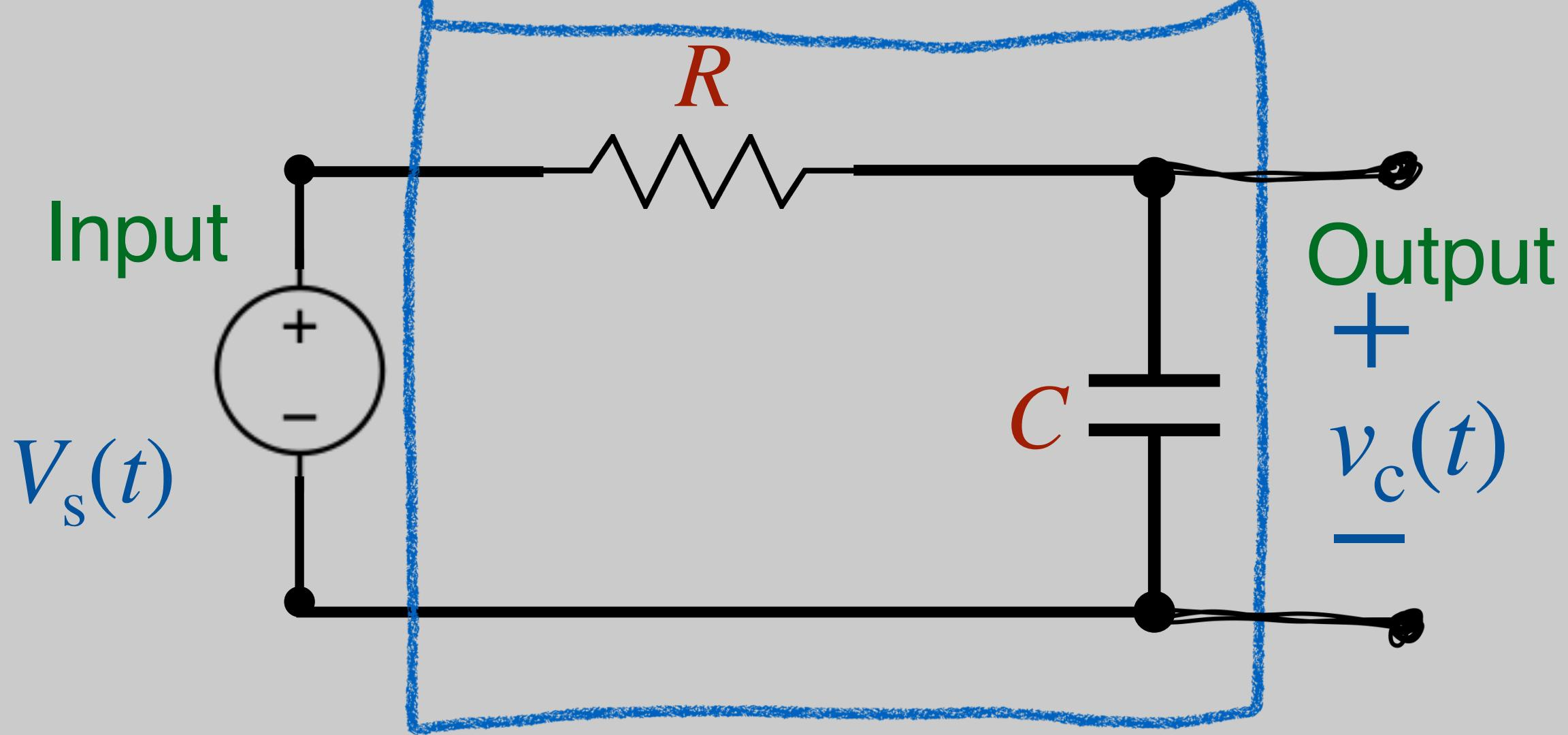
Solution:  $v_c = V_0 \left( 1 - e^{-\frac{t-t_0}{RC}} \right)$
