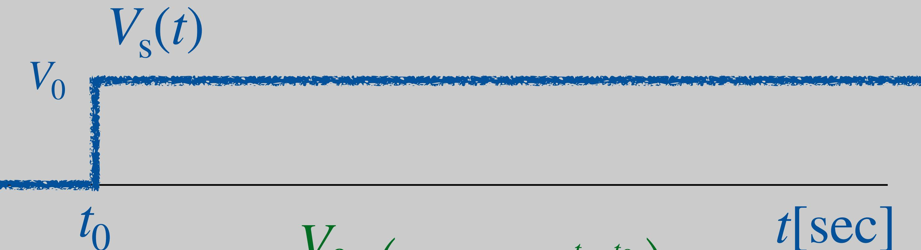
$$i_L = \frac{V_0}{R} \left( 1 - e^{-L\frac{t-t_0}{R}} \right)$$
