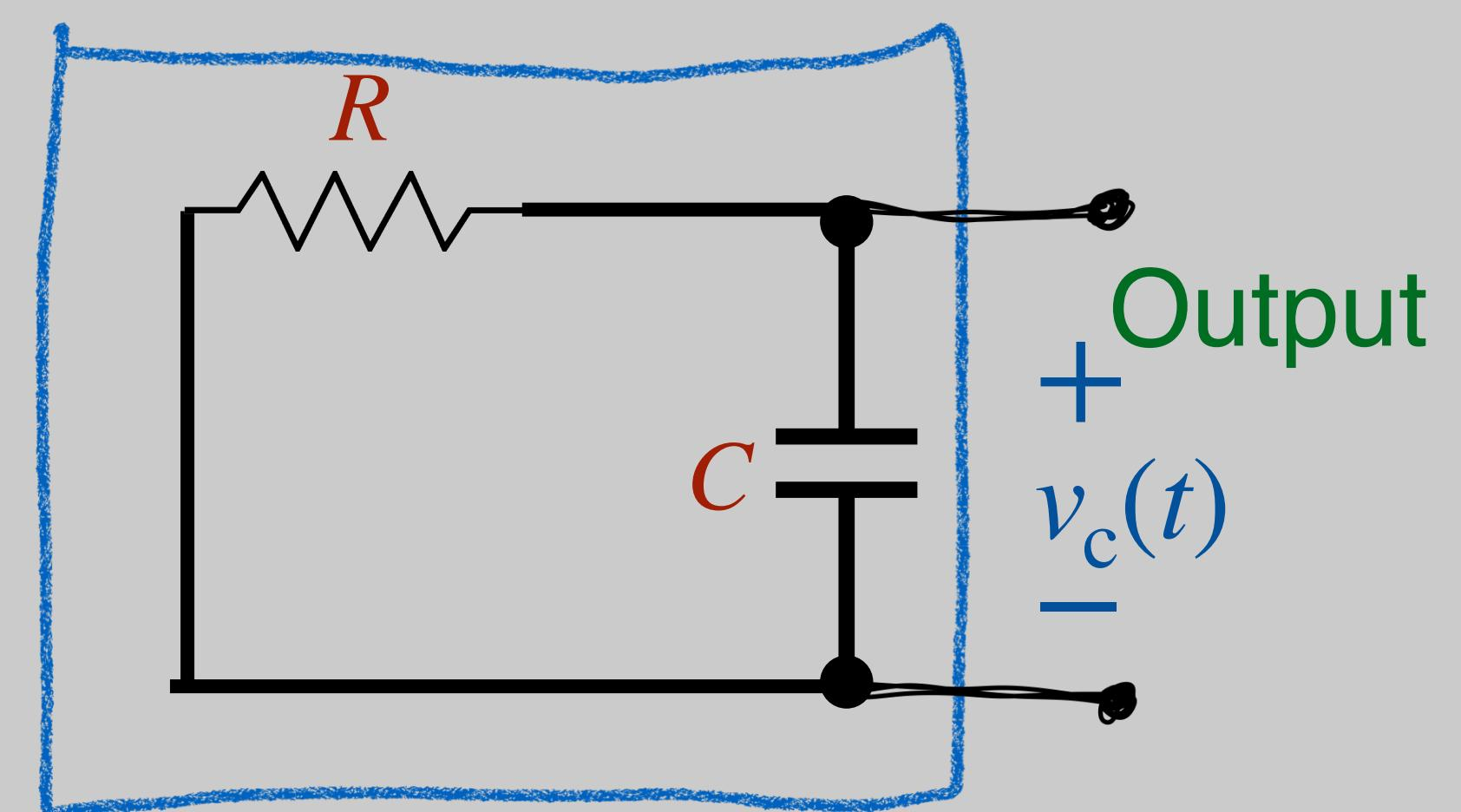
Solution:  $v_c(t) = V_0 e^{-\frac{t}{RC}}$
