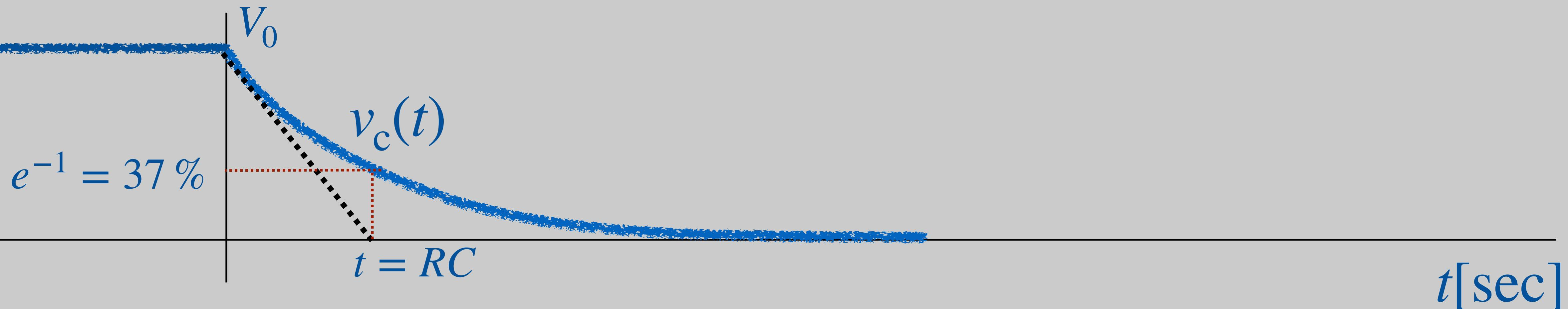
$$RC \rightarrow [\Omega][F] = \frac{[V]}{[A]} \frac{[C]}{[V]} = \frac{[C]}{[A]} = \frac{[C]}{[C]/[s]} = [s]$$
