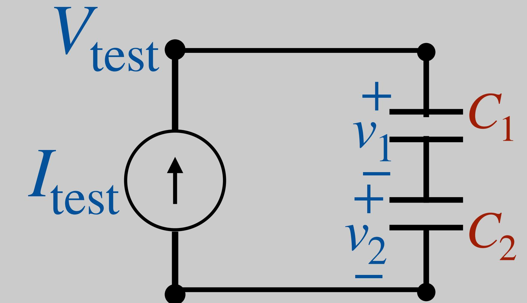
$$i_{\text{test}} = C_{\text{eq}} \frac{dV_{\text{test}}}{dt} = C_{\text{eq}} \frac{dV_1}{dt} + C_{\text{eq}} \frac{dV_2}{dt}$$
