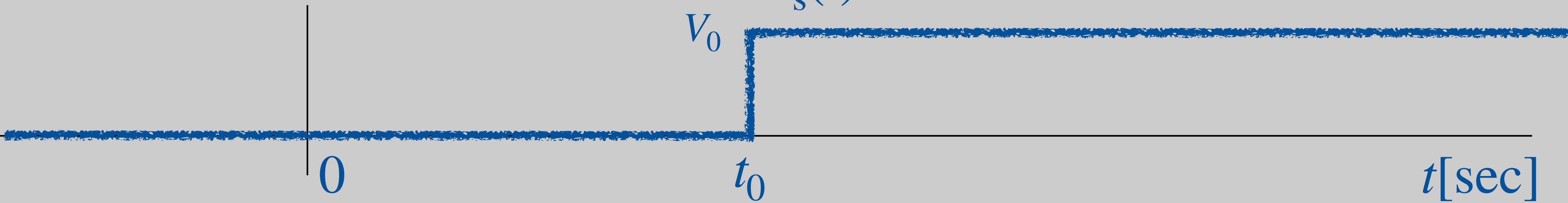
$$V_s(t) = V_0 \quad |t > t_0$$
