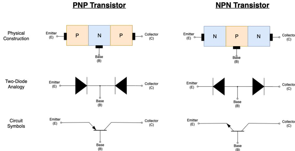
Let's now explore how we can bias this component so we can use it as a switch. We want the current between the collector and the emitter to be controlled by the current between the emitter and the base.
