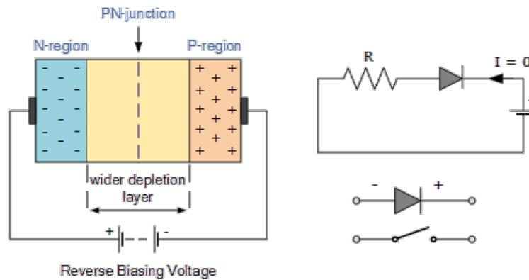
In the reverse-biased case, the external voltage is applied in the same direction as the barrier voltage, so it adds to the barrier voltage, making the effective barrier voltage the sum of the open-circuit barrier voltage and the applied voltage. This makes it much more difficult for electrons and holes to diffuse across the depletion region, so the device allows only a very small amount of current to flow: for the ideal diode abstraction, we consider this current to be 0.
