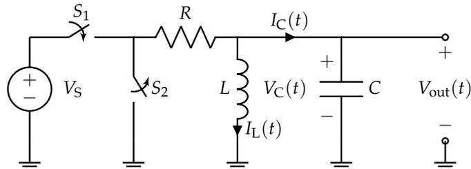
The switch  $S_1$ , open for  $t < 0$ , closes at  $t = 0$ , and the switch  $S_2$ , closed for  $t < 0$ , opens at  $t = 0$ . Assume  $V_C(0) = 0$  and  $I_L(0) = 0$ .
